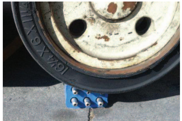
Adapter pins were fully functional after testing even though the pins were not supported by a plug assembly when the 2500 pound load was applied.
